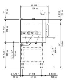
CWI1 = Cold Water inlet 1 (cleaning) CWI2 = Cold Water Inlet 2 (steam
